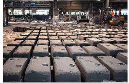
Sand Molds Ready for Pouring Molten Metal
