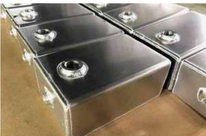
Fabricated hydraulic tanks
