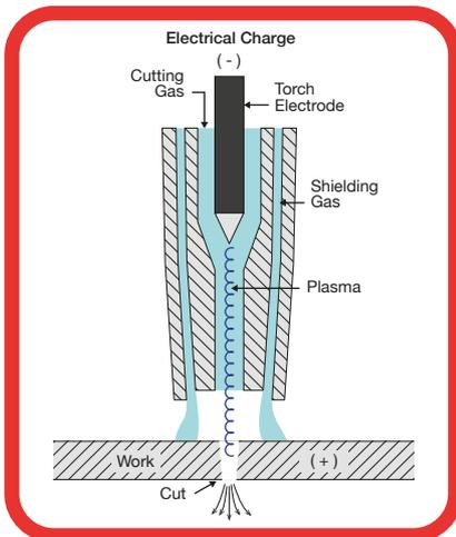
Plasma Cutting is a thermal-based process that uses a jet of super-heated plasma to cut through electrically conductive materials (including steel, aluminum, brass and copper).
